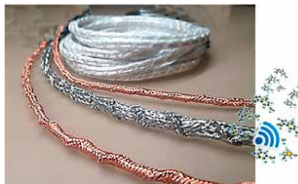
Fig. 16: ... for cable humidity sensors in concrete
