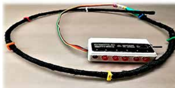
Fig. 10: Six-zone cable humidity sensor with indicator unit for critical excess of humidity in the control zones
